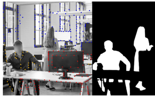
Fig. 5. Vision-based traversability prediction is an open problem in crowded office environments where occlusions and obstacles are rich. In a crowded dynamic scene, it is difficult to obtain a good point cloud map and human detection due to occlusions and obstacles. The left and right panels show the DSO point cloud map and Detectron2 human detection mask, respectively.
